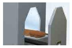
Samples to be measured for colour are in the DigiEye Cube, which excludes ambient light in favour of controlled, consistent lighting to a standard close to CIE D65. Different illumination geometries are possible, including angled and diffuse lighting.
